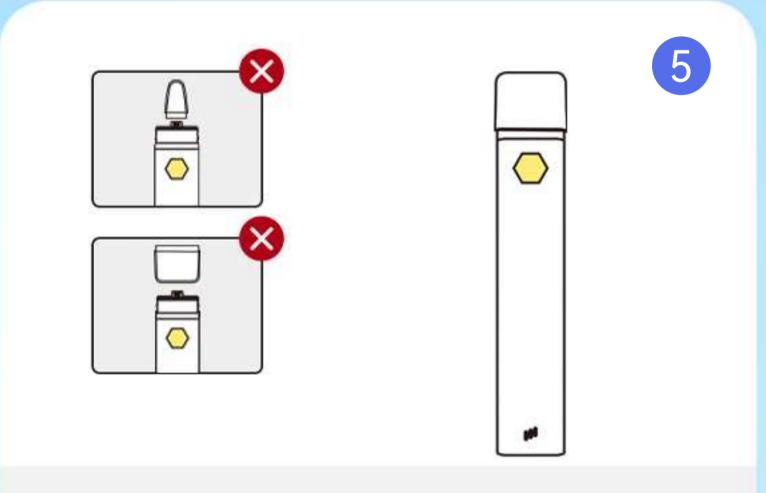
When snapping in the mouthpiece, it should be vertical to the device and forced evenly.
