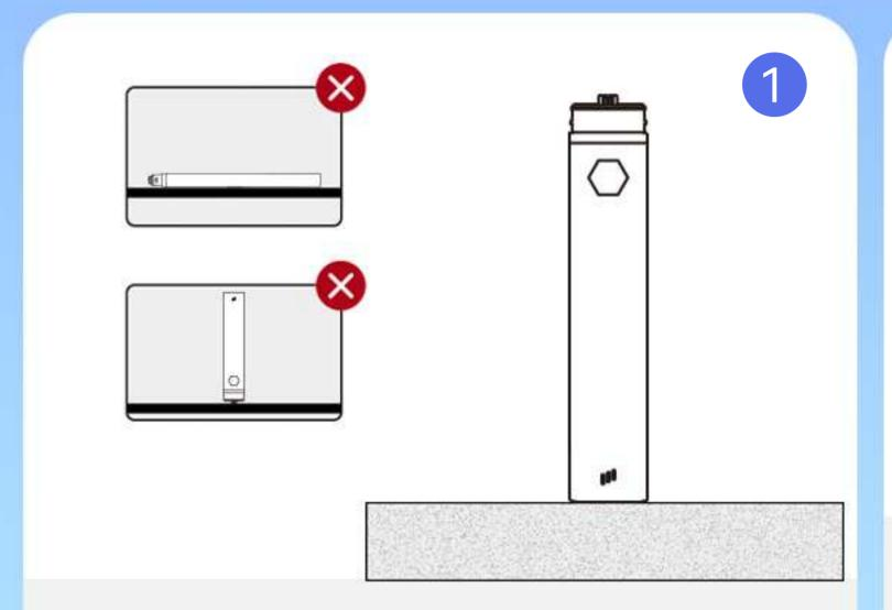
• Unpackge the cartridge and make sure it is vertically upright with the tray.
