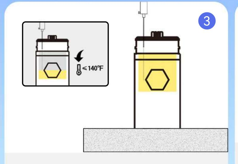
• The output temperature must be under 140°F.
