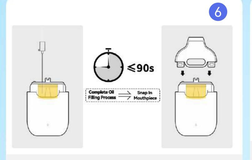
Complete the snapping process within 90s after filling the oil.
