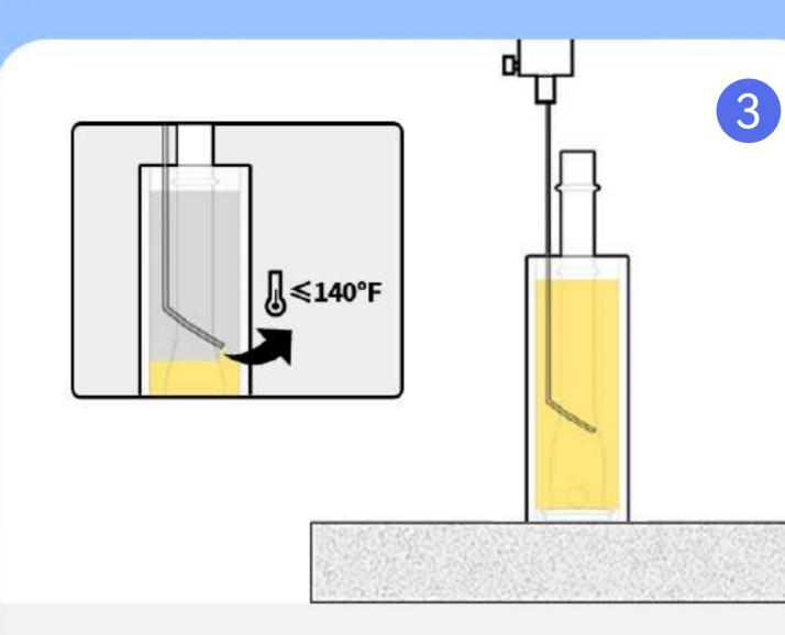
• The output temperature must be under 140°F.
