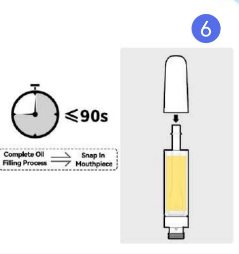
Complete the snapping process within 90s after filling
