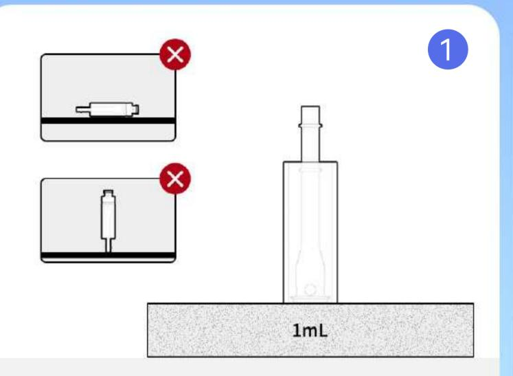
• Unpackge the cartridge and make sure it is vertically upright with the tray.
